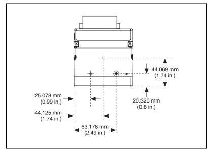
Figure 4. NI 9144 Chassis, Side View with Dimensions
